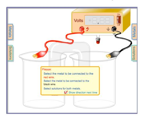
This simulation contains an apparatus for measuring the voltage generated by chemical reactions. This apparatus is called a voltaic cell. Pop out menus will allow you to select metals (electrodes) and ionic solutions to be placed into two beakers that are connected by a salt bridge. You can then connect the metals to a voltmeter to measure the cell voltage (E°).
