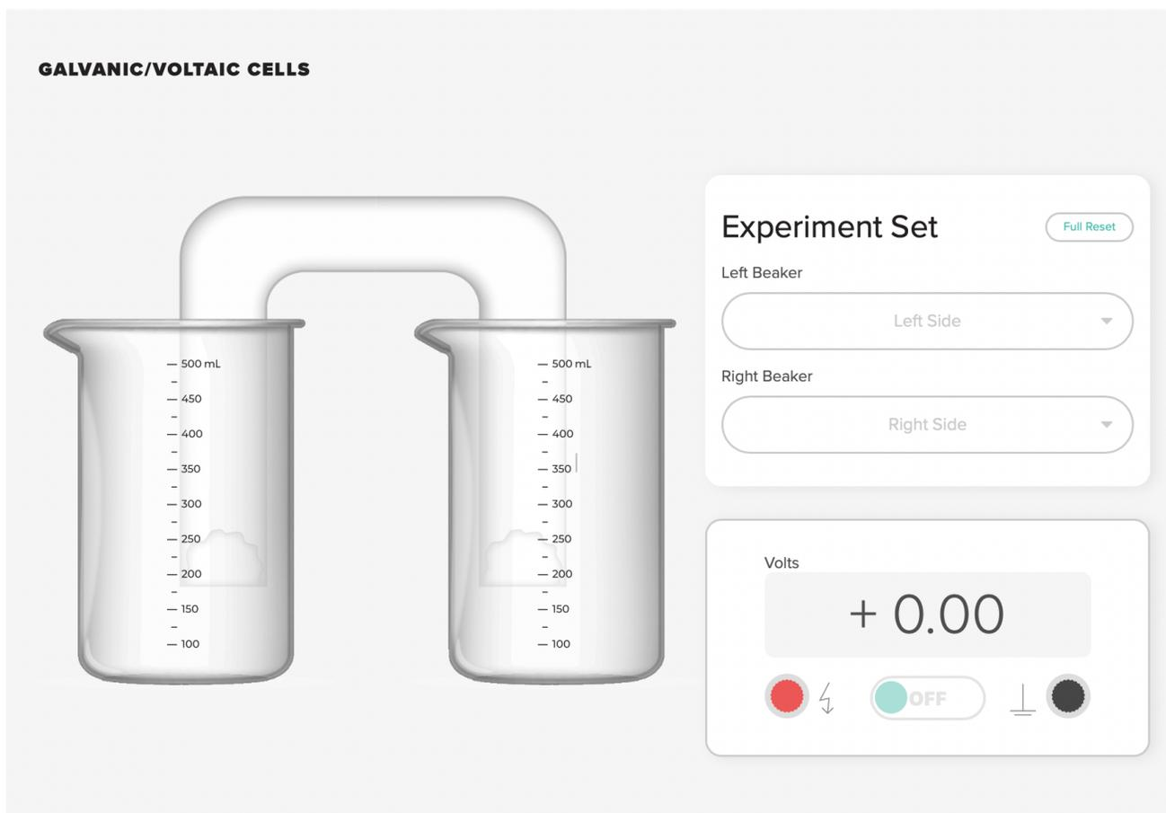
This simulation contains an apparatus for measuring the voltage generated by chemical reactions. This apparatus is called a voltaic cell. Pop out menus for the Left Side electrode and for the Right Side electrode will allow you to select metals (electrodes) and ionic solutions to be placed into two beakers that are connected by a salt bridge. You can then connect the metals to a voltmeter to measure the cell voltage ( $E^\circ$ ).
